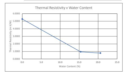
Notes: Water content measured in accordance with ISO 17892-1:2014. Bulk density measured by linear measurement. Porosity calculated (voids ratio/1+voids ratio) with an assumed Particle Density of 2.65. Thermal measurements undertake using a TEMPOS and TR-3 probe (manufactured by METER Group). \*Thermal test results are an average of 5 readings.
