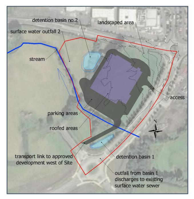
Figure 4-1 Schematic Layout of Proposed Development
