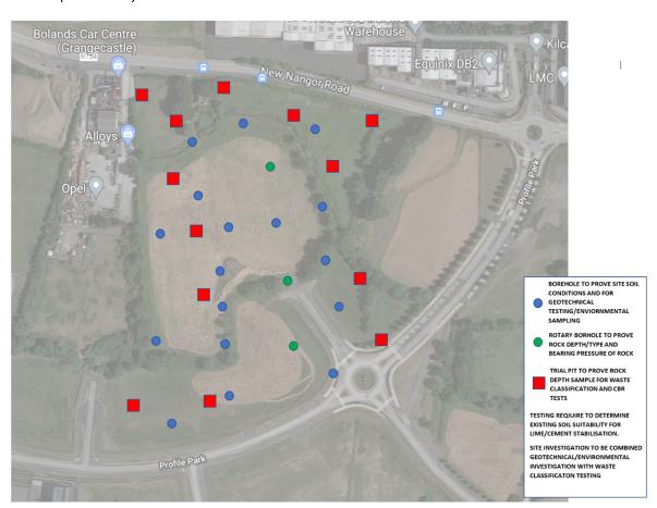
Refer attached for a site plan indicating trial pits, borehole and CBR test locations - could you provide us with a price and programme to undertake the site investigation works to include for the following:-
