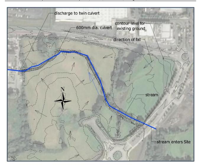
Figure 3-2 Site Topography / Main Drainage Features
