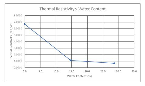
Notes: Water content measured in accordance with ISO 17892-1:2014. Bulk density measured by linear measurement. Porosity calculated (voids ratio/1+voids ratio) with an assumed Particle Density of 2.65. Thermal measurements undertake using a TEMPOS and TR-3 probe (manufactured by METER Group). \*Thermal test results are an average of 5 readings.
